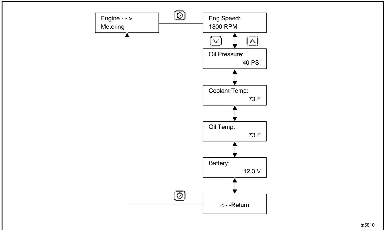
Figure 23 Engine Metering Menu
