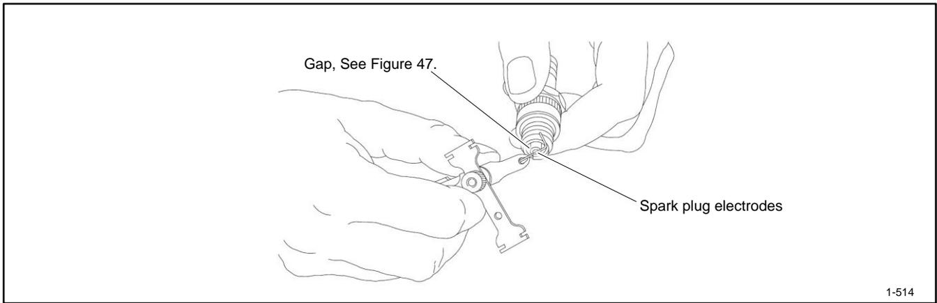
Figure 48 Spark Plug Gap Inspection
