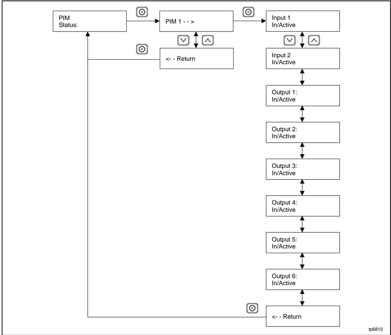
Figure 36 Programmable Interface Module (PIM) Status Menu
