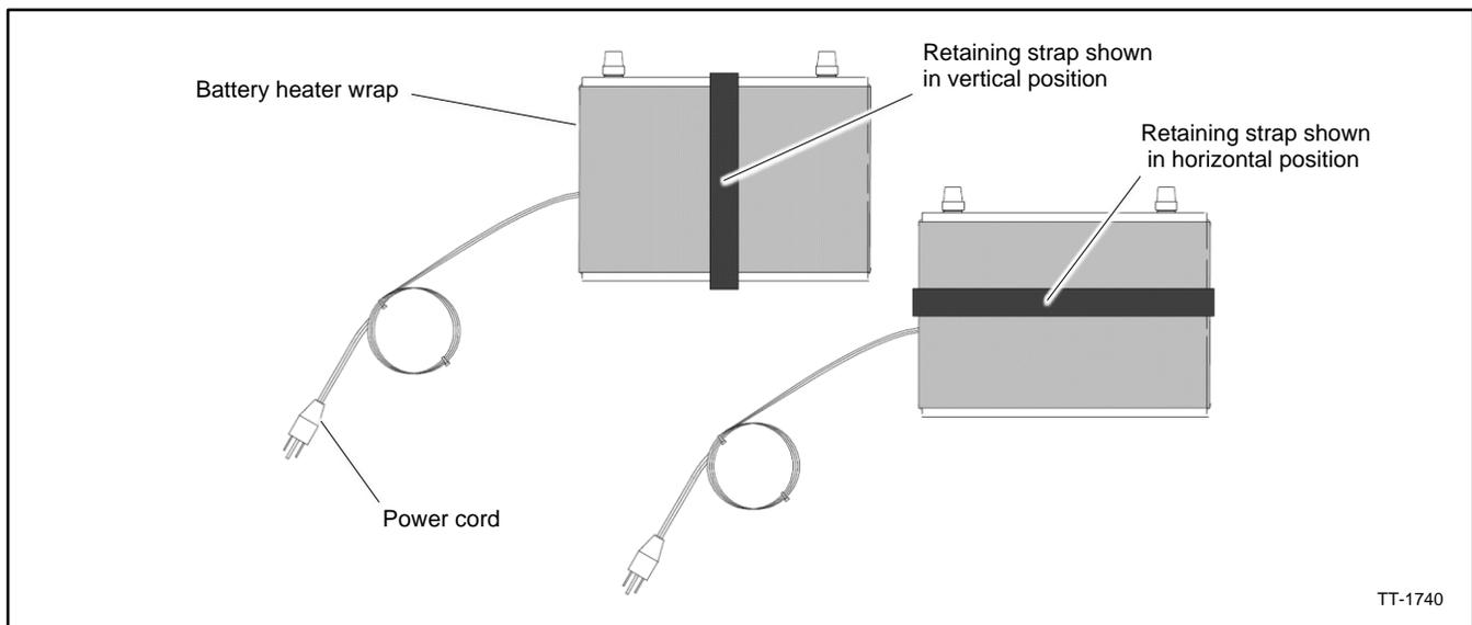
Figure 39 Typical Battery Heater
