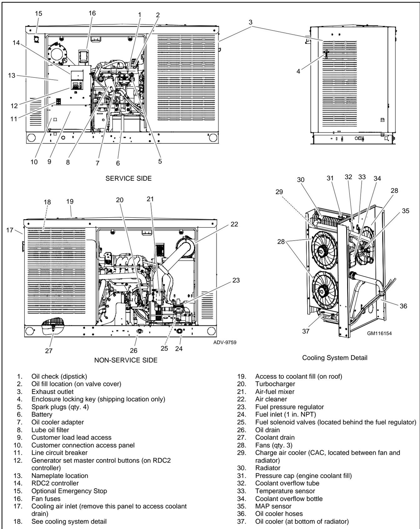
Figure 5 30RCLA and 38RCLC Service Views for Maintenance
