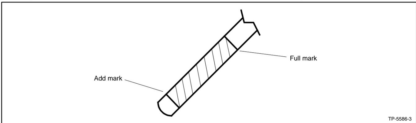
Figure 42 Oil Level Check
