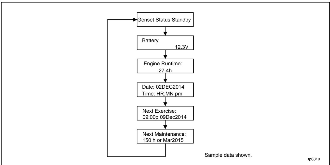
Figure 19 Autopaging Displays, Automatic Mode
