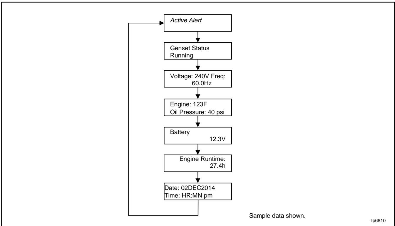
Figure 18 Autopaging Displays, Generator Running
