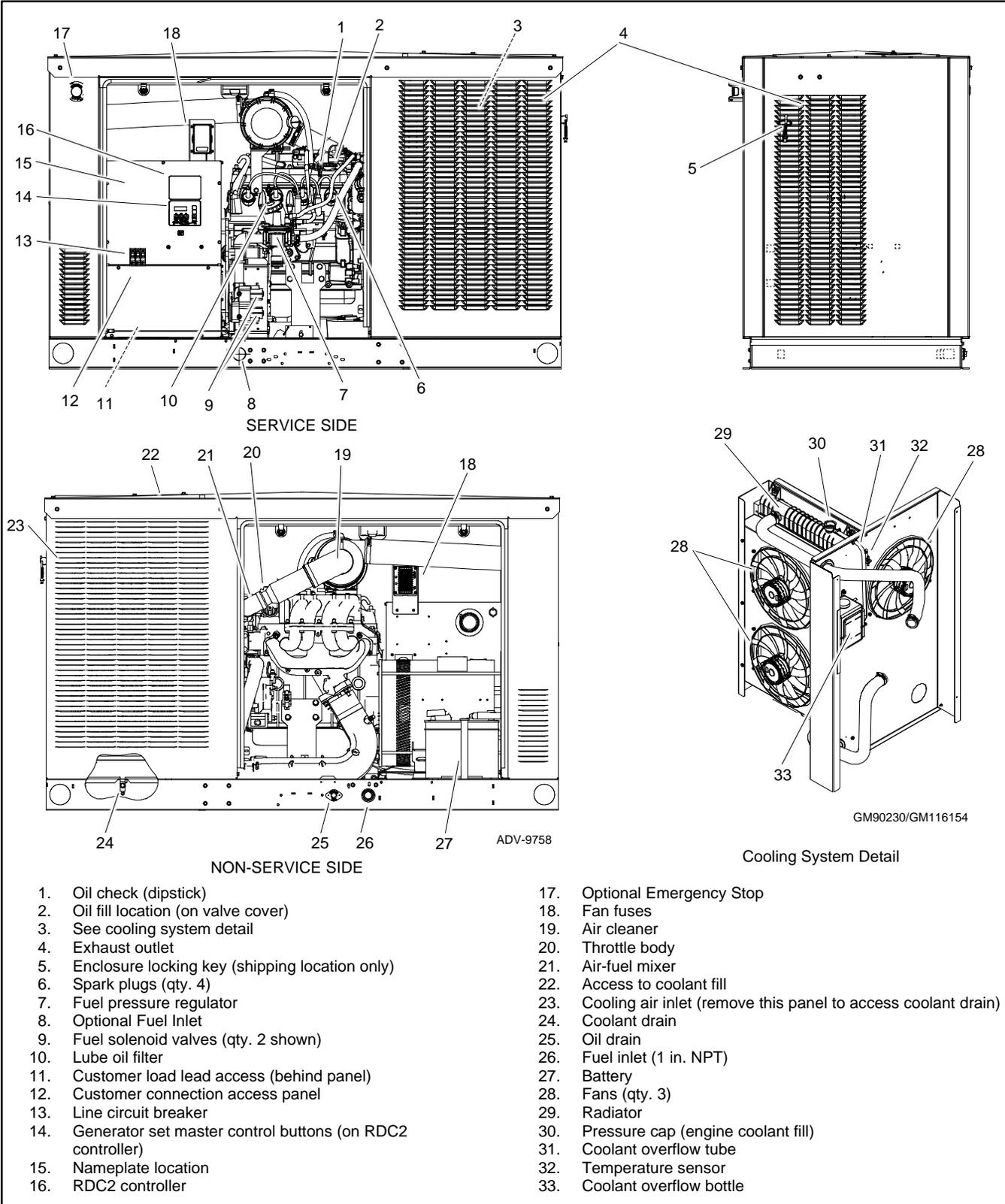
Figure 4 24RCL/RCLA Service Views for Maintenance
