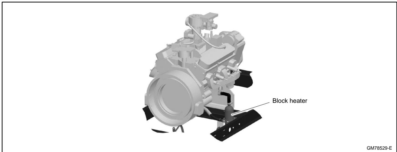
Figure 40 Block Heater (typical location)
