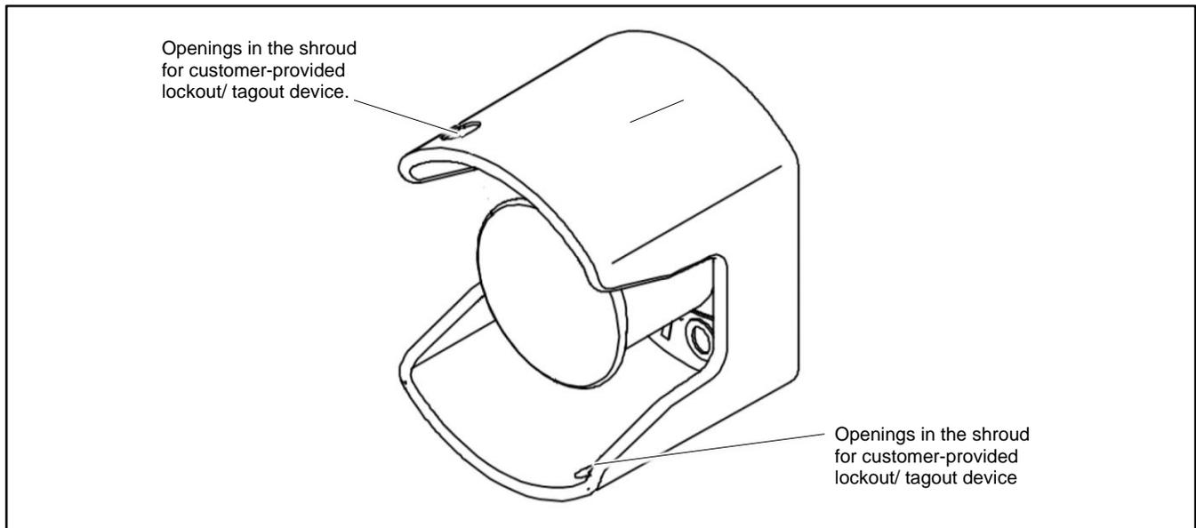
Figure 41 Emergency Stop Switch (typical)
