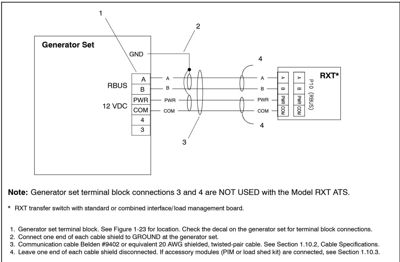
**Figure 1-27** Model RXT Transfer Switch Communication Connection to Generator Set Terminal Block
