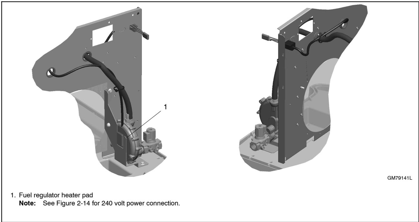
**Figure 2-15** Installed Regulator Heater Kit (for 20RESA/RESAL/RESC/RESCL)
