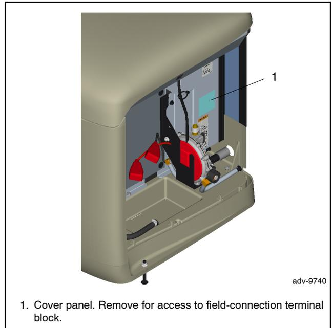
**Figure 1-23** Field-Connection Terminal Block Location
