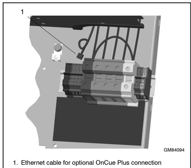
Figure 2-6 Network Connection for OnCue Plus
