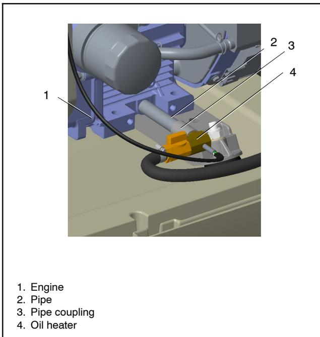
**Figure 2-22** Oil Heater, Typical
