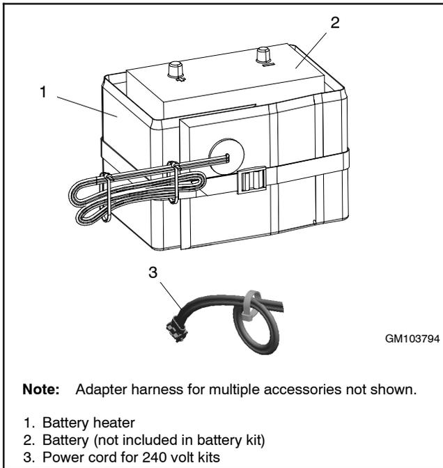
**Figure 2-17** Battery Heater
