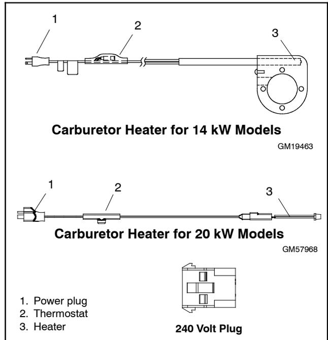
**Figure 2-9** Carburetor Heaters
