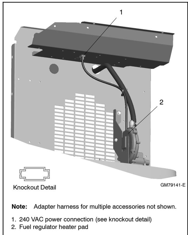
**Figure 2-14** Model 20RESA/RESAL/RESC/RESCL 240 Volt Kit Power Connection
