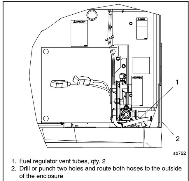
**Figure 1-20** Fuel Regulator Vent Hoses (20 kW only)
