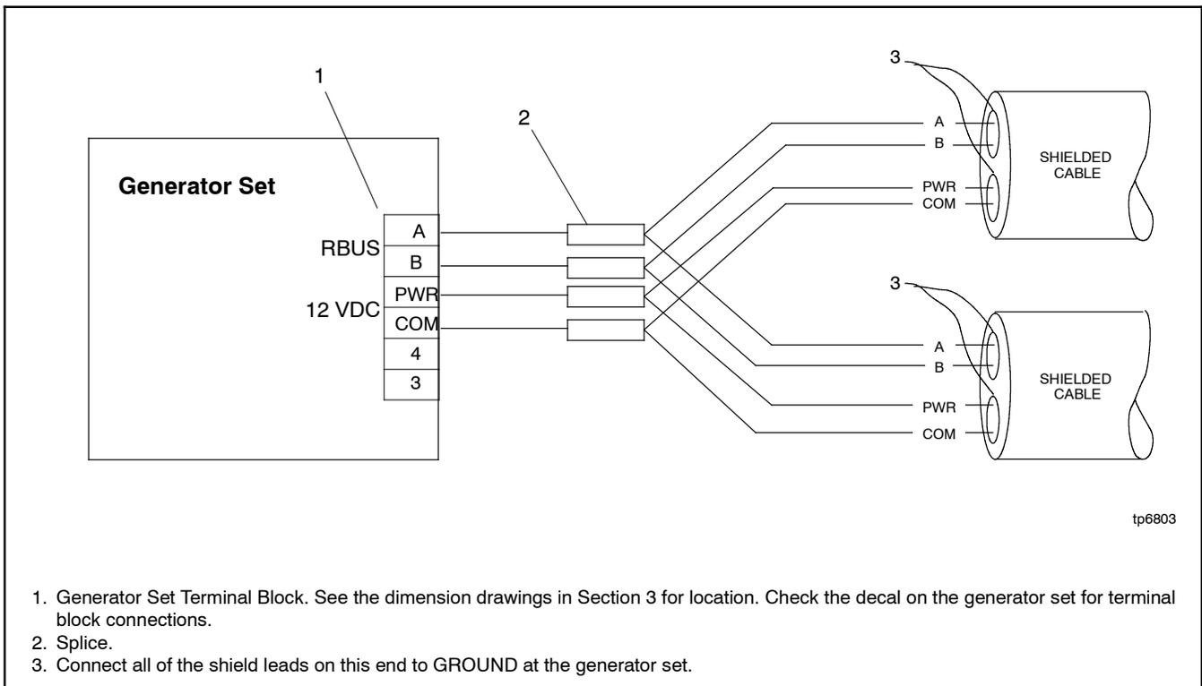
**Figure 1-33** Multiple Connections to the Generator Set
