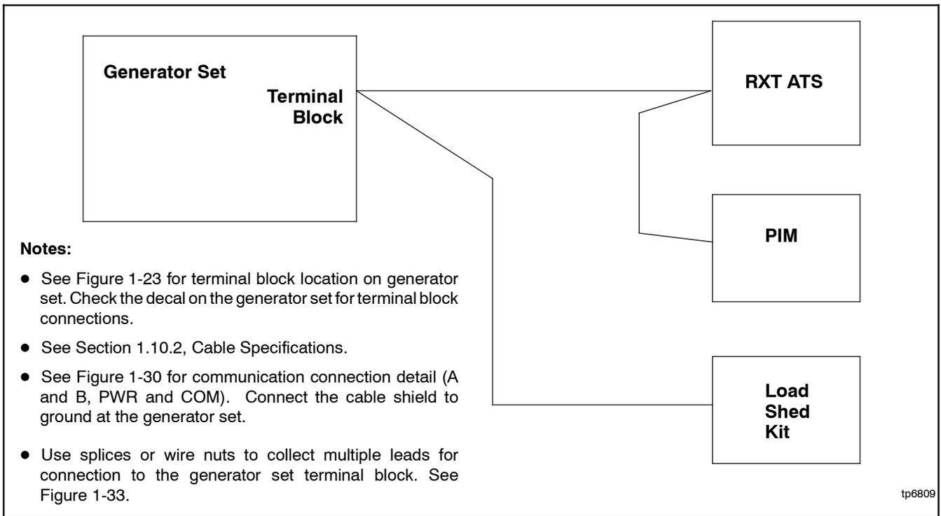
**Figure 1-34** Accessory Module Connections (two cable runs with one and two modules shown)
