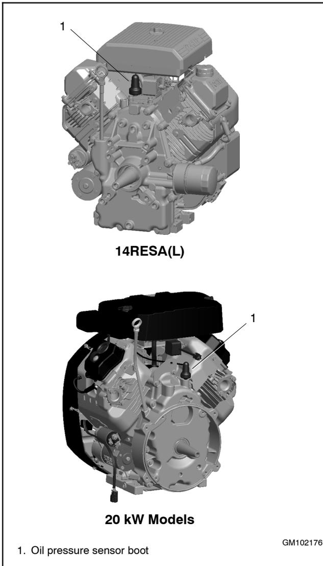
**Figure 2-24** Oil Pressure Sensor Boot Location
