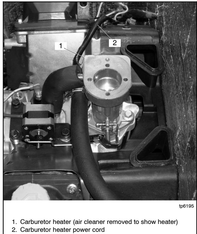
**Figure 2-10** Carburetor Heater for 14 kW Models
