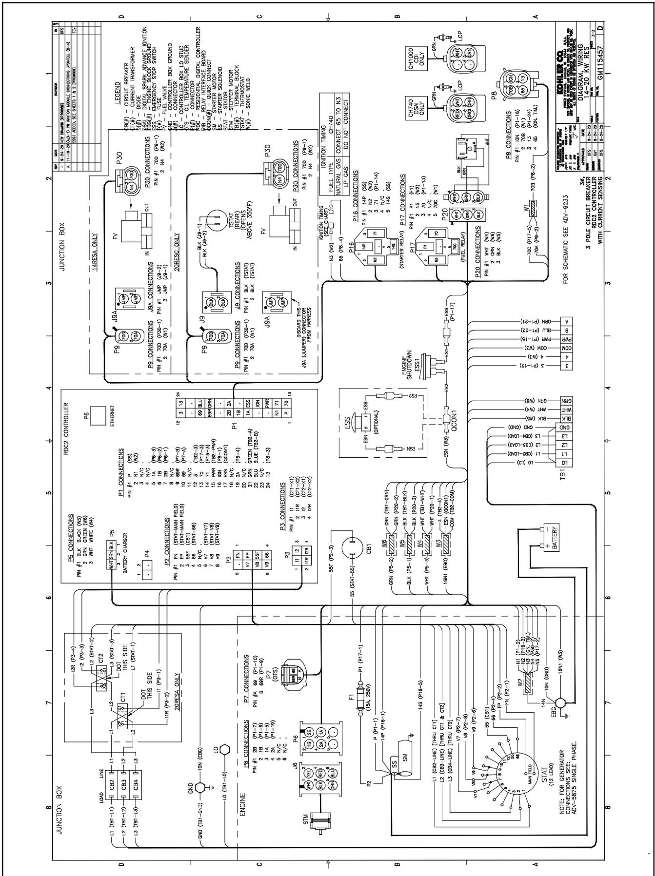
Figure 3-16 Point-to-Point Wiring Diagram, 14RESA(L) and 20RESC(L), GM115457, Sheet 3 of 3
