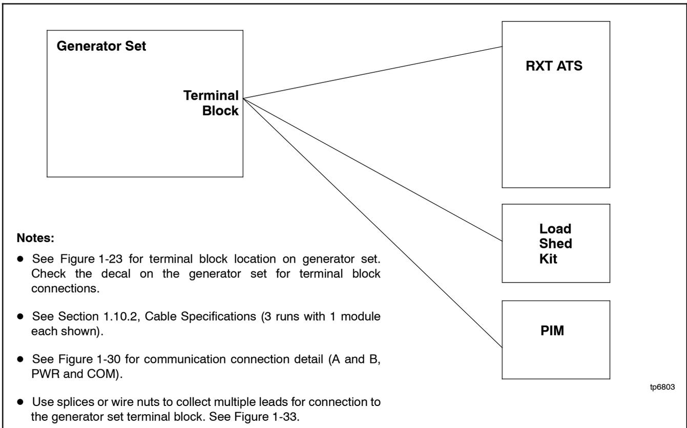
**Figure 1-32** Accessory Module Connections (three cable runs with one module each)
