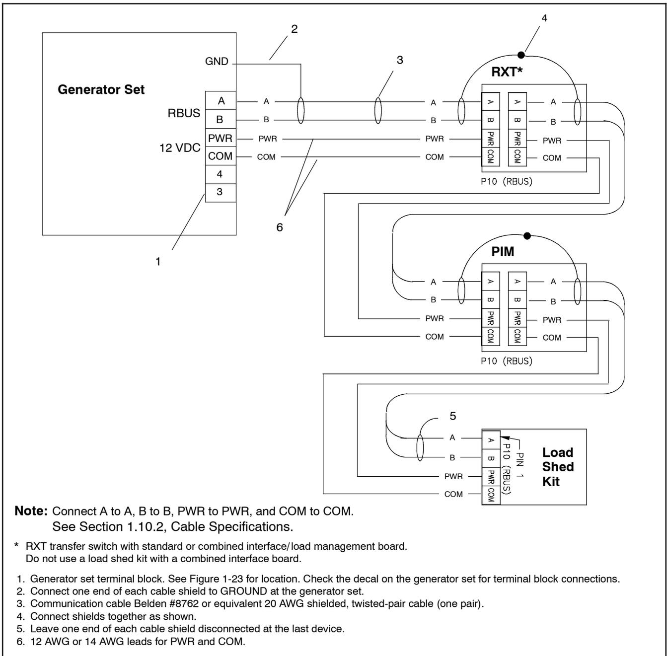
**Figure 1-31** Accessory Module Connections with 12- 14 AWG Power Leads
