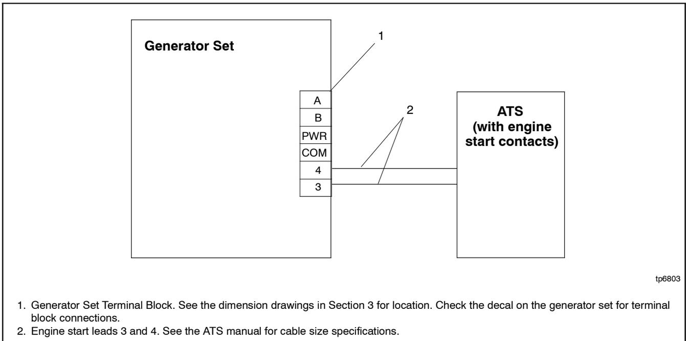
**Figure 1-28** Engine Start Connections with Transfer Switch Models other than Model RXT
