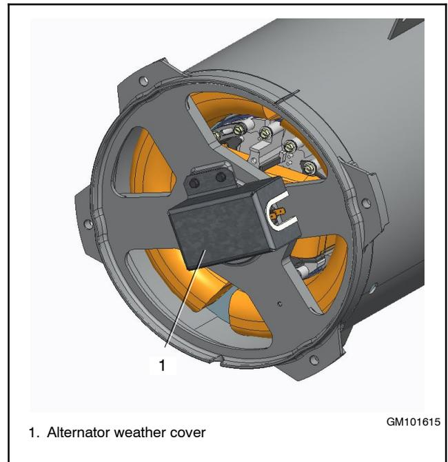
**Figure 2-23** Alternator Weather Cover
