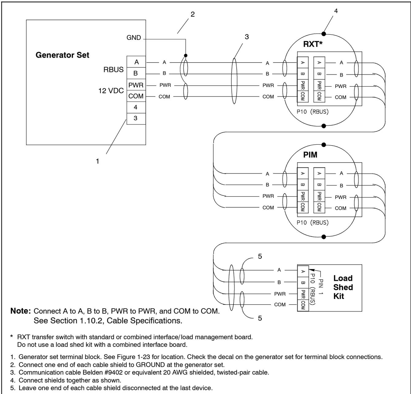
**Figure 1-30** Accessory Module Communication Connection Details
