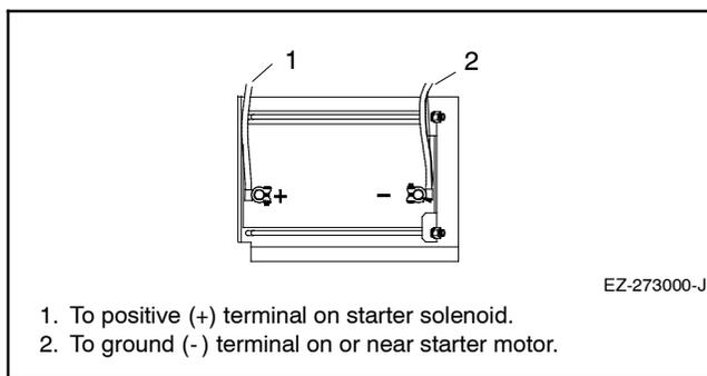
**Figure 1-35** Typical Battery Connection
