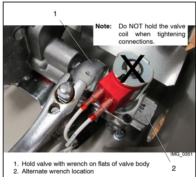
Figure 1-8 Holding Fuel Valve to Tighten Fuel Connections (Original Fuel System Shown)
